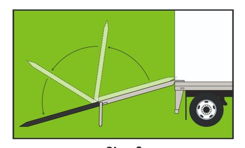
**Step 6**Unfold ramp, resting it on ground
